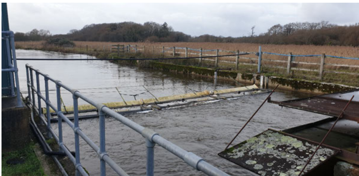
Figure 2. Floating PIT tag array on the River Frome. Upstream of this array is the acoustic bubble screen used to divert smolts into a side channel.
